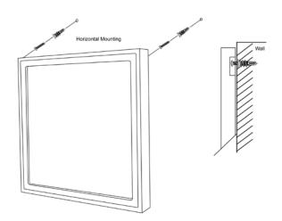
Note: If either mark happens to align with a wall stud (use a stud finder to determine this), do not use the provided anchors because they cannot penetrate wood. If a mark does align with a stud, only use one of the provided screws at this mark. Use the screwdriver to secure a screw at the mark directly into the wall and stud. Rotate the screw clockwise until the screw head is about 3/8" from the wall.
