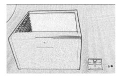
2) Now position the handle as shown below. The handle is inserted into the front slot of the box so that it projects upwards (when the box is upright). The hole in the handle should align with the hole in the box. Insert the bolt through both the box hole and the handle hole and secure the nut to the bolt. Tighten using the tools.
