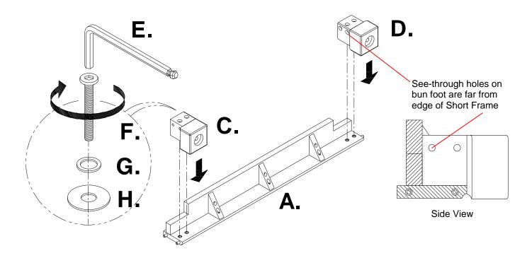
2. Align and attach the assembled Short Frames to each end of a Long Frame (B). Insert bolts with washers through pre-drilled holes located on the bun foot into insert nuts located on the Long Frame (B). Repeat with the other Long Frame (B). Check alignments and fully tighten all connecting bolts.
