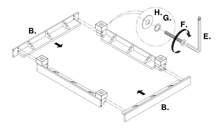
3. Turn levelers located on bottom of feet in and out to keep the base level when needed.
