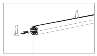
1. Attach hangers to the tubes by inserting into the tubes' channels (evenly spaced apart).
