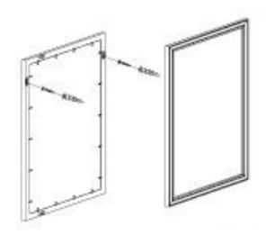
4) Preferably with the help of another person, lift the item so that the two selected keyholes align with and engage the protruding screw heads. Gently lower the item so that the screws support its full weight. Make sure that each screw is completely engaged with its keyholes before releasing the item.
