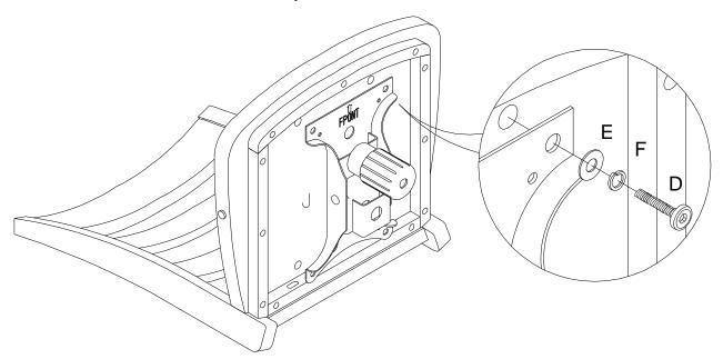
4. To attach Chair Seat (A) to the Chair Base (B), align and connect the hole in center of the Metal Bracket at bottom of the Chair Seat onto the assembled Cylinder (G) on the Chair Base. Firmly apply pressure onto the Chair Seat with both hands to ensure chair slides onto the Cylinder (G).
