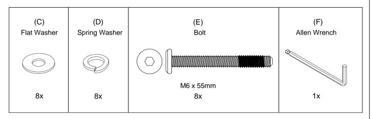
Attach Leg (B) to Top Panel (A) as shown, insert Bolt (E) thru Spring Washer (D) and Flat Washer (C) and tighten with Allen Wrench (F).
