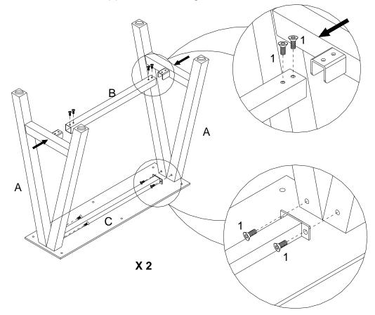
2. Secure the Metal Plate(C) to A Frames(A) using bolts(1), tighten by hand at first, securely tighten the bolts with Allen wrench(5), but do not over tighten the bolts.
