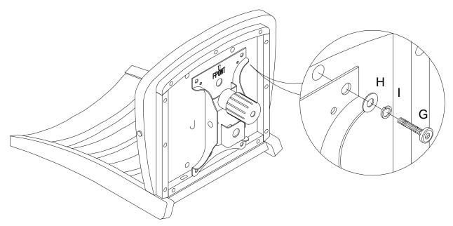
4. Slide a Spring Washer (I) and a Flat Washer (H) onto each Long Bolt (F). Attach Left Arm Rest (C) to the Chair Seat and insert a long bolt with washers from arm rest into insert nuts to the seat panel. Place a Barrel Nut (J) onto opening under the arm rest and insert a long bolt with washers from post of the chair seat to secure. Repeat with the Right Arm Rest (D). Check alignments and fully tighten all connecting bolts.
