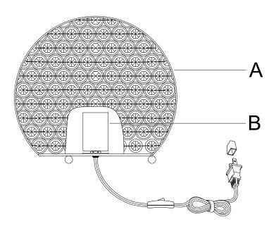
Insert the specified light bulb into the Socket (B). DO NOT EXCEED THE SPECIFIED WATTAGE.
