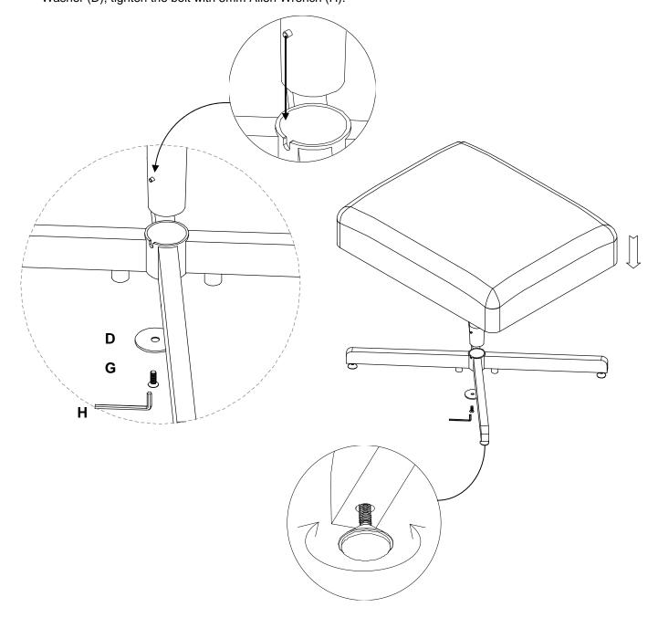
4. Adjustable levelers are installed to accommodate uneven flooring. To adjust these levelers, simply turn them clockwise to up or counterclockwise to down. Assembly is complete!
