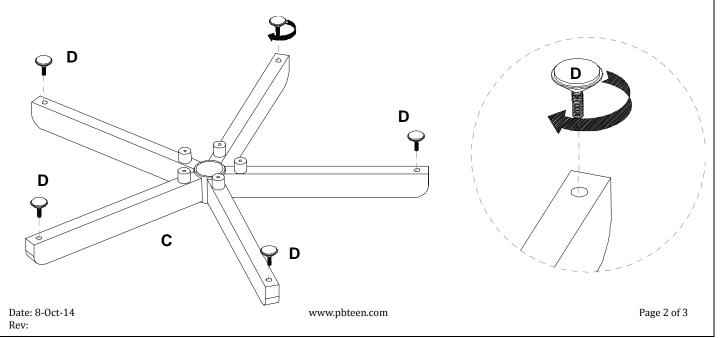
2. Insert Post (B) into Base (C) by pressing firmly. Adjustable levelers are installed to accommodate uneven flooring. To adjust these levelers, simply turn them clockwise to up or counterclockwise to down.
