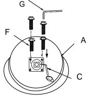
Step4. Put Seat (A) to Gas Lift Post (D) by pressing firmly with Seat plate (C).
