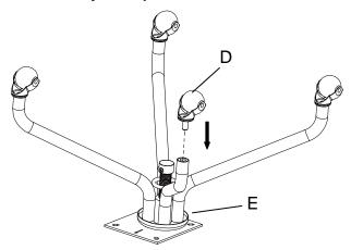
2. Attach Base (E) to the bottom of Seat (C) as shown (**NOTE: the arrow on the Base should towards the long side of the Seat**), insert Bolt (F) and tighten with 4mm Allen Wrench (I).
