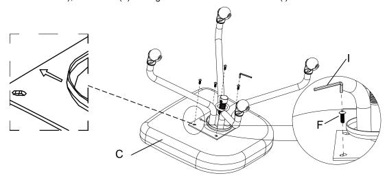
3. Attach Metal Frame (B) to the Seat (C) as shown, insert Allen Head Bolt (G) and tighten with 5mm Allen Wrench (J).
