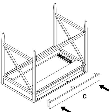
8. Secure the rail from inner side of drawer box by using Bolt (I), Spring Washer (G) and Flat Washer (F), tighten with Allen Wrench (J).
