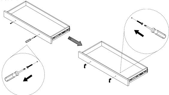
10. Pull out the inner rail of the slide on drawer box out to the maximum extent. Align the slide on drawer with the slide on drawer box as shown, push drawer into the box. Push and pull the drawer back and forth a few times until it is locked firmly.
