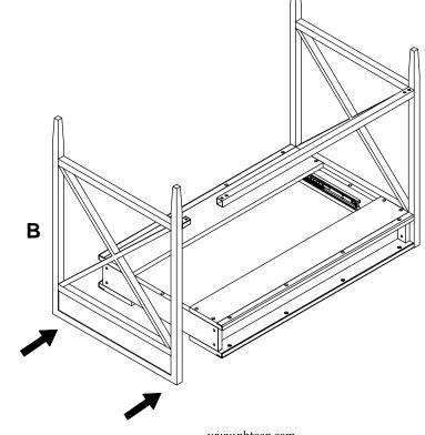
5. Secure the bottom rail with Bolt (H), Spring Washer (G) and Flat Washer (F), tighten with Allen Wrench (J).
