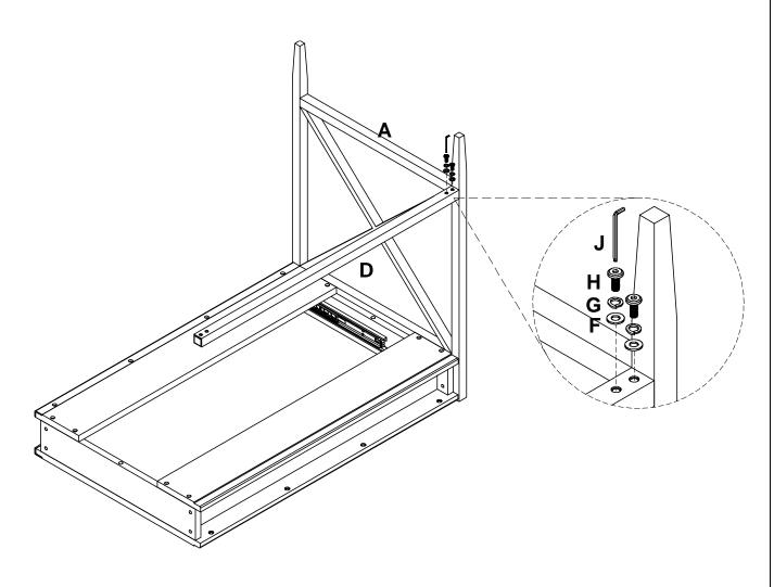
4. Attach Right Frame (B) to the assembly as shown.
