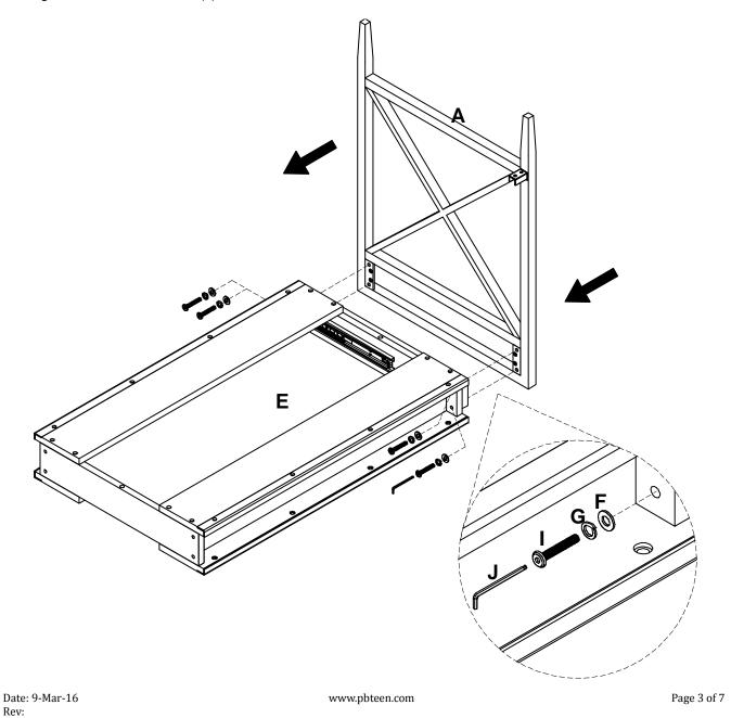
3. Attach Bottom Rail (D) to Left Frame (A) as shown, insert Bolt (H) thru Spring Washer (G) and Flat Washer (F), tighten with Allen Wrench (J).
