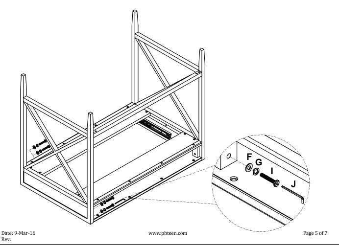
7. Attach Top Rail (C) to the assembly as shown.
