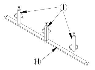
4 of 7 www.pbteen.com 7. Attach this assembled Supporting Rail (H) and Support Leg (I) with Slats Roll (G). Connect the 1<sup>st</sup> slat to the end of Supporting Rail (H). This can be done by inserting Hex Bolt (L) followed with spring washer (M) and flat washer(N) through the pre-drilled hole in 1<sup>st</sup> slat, and into the pre-drilled holes in Supporting Rail (H). Tighten with Allen Key (K). Repeat at the other end.
