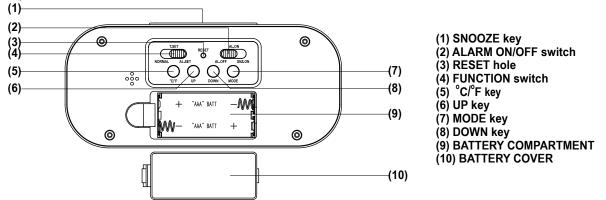
At first, open the **BATTERY COVER (10)** and insert 2 x 'AAA' size batteries into the **BATTERY COMPARTMENT (9)** as the polarity indicated, then close the **BATTERY COVER (10)**.
