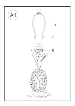
Raise the Harp Caps (F) and insert the bottom ends of Harp (B) into the Saddle (E)
