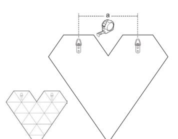
With the back of the item facing away from the wall, hold it against the wall at a desired mounting location. Mark two reference points (A, B) on the wall as shown.
