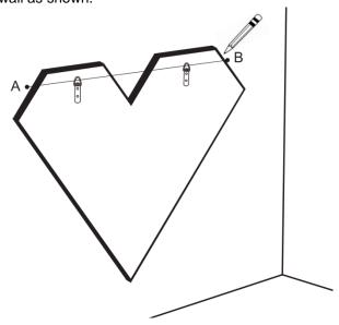
3 Connect the two points (A, B) with a light pencil line. Use a level to ensure that the line is level.
