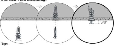
The anchor is self-drillable. No pilot hole required.
