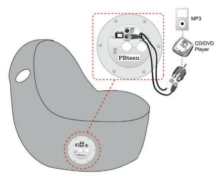
**3.** Turn the power switch (A2) to on position, and raise or lower the volume or bass with the knobs located on the control panel (A4, A5).
