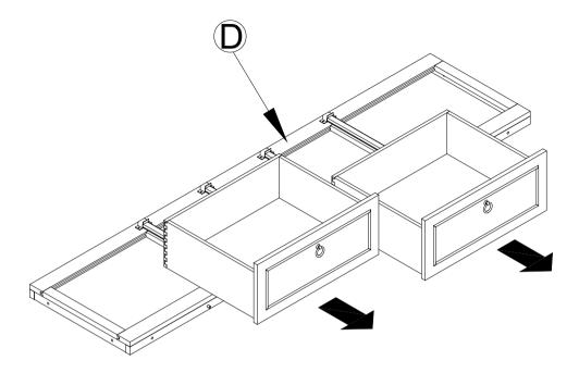
2. Attach the Drawer Boxes (D) bottom panels to the Siderails (C) as shown below. Place the Flat Washer (N), Spring Washer (M) and followed by the Short Allen Bolt (L) – 3sets; into the pre-drilled holes of the Drawer Boxes (D) bottom panel into the Siderails (C) and tightening using the Ball Tip Allen Ley (H) as shown below.
