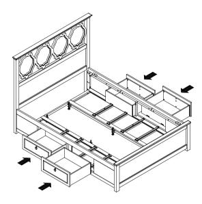
9. Lay the Slats (E) on top as shown below. Secure the Slats (E) by inserting the the Long Philip Headscrew (O) into the pre-drilled holes of each Slats (E). Tighten using the Philip Screwdriver (Not Included).
