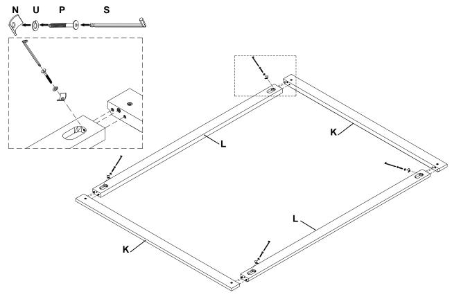
8. Place Canopy assembly the post and attach it by inserting Allen Bolt (P) from the top and tighten with Allen key (S) as shown below.
