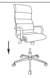
Step 5: Put the assembled upper part to the assembled base part.
