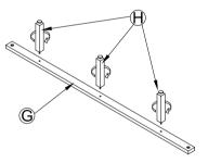
10. Place the Slats Support Strecther (G) afix with the Slats Support Legs (H) onto the surface floor in between the Bed as shown below.
