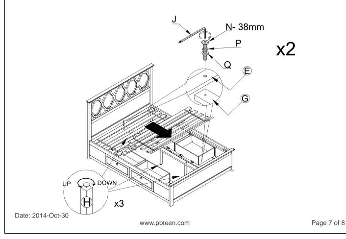
13. Secure the Slats (E) by inserting the the Long Philip Headscrew (R) into the pre-drilled holes of each Slats (E). Tighten using the Philip Screwdriver (Not Included).
