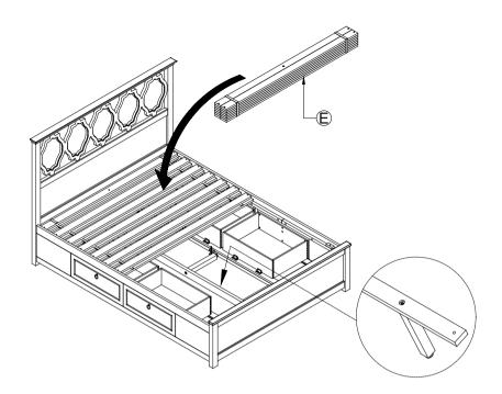
12. Attached the Slats Support Strecther (G) afix with the Slats Support Legs (H) to the pre-drilled holes of the Slats (E) by placing the Flat Washer (Q), Spring Washer (P) and followed by Medium Allen Bolt (N) on the center surface of the pre-drilled holes of Slats (E). Tighen it by using the Ball Tip Allen Key (J). After fixing on the 1<sup>st</sup> Medium Allen Bolt (N), fully extend the Slats (E). Illustration as shown below.
