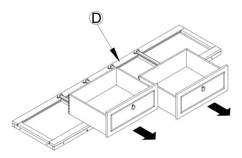
2. Attach the Drawer Boxes (D) bottom panels to the Siderails (C) as shown below. Place the Flat Washer (Q), Spring Washer (P) and followed by the Short Allen Bolt (O) – 3sets; into the pre-drilled holes of the Drawer Boxes (D) bottom panel into the Siderails (C) and tightening using the Ball Tip Allen Ley (J) as shown below.
