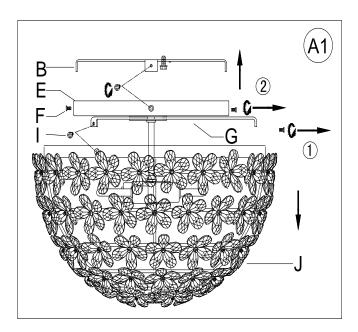
1. Separate the Canopy (E) from the Frame (J) by removing the 3 Frame Screws (I) anti-clockwise
