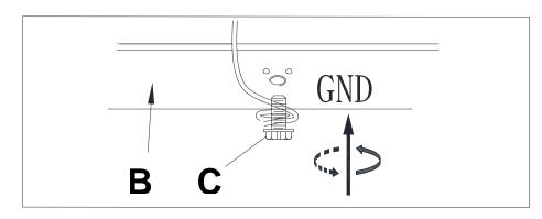
If junction box DOES NOT has a GROUND WIRE, wrap the fixture's bare ground wire around the Green Ground Screw (C) and insert the screw into the Mounting Plate (B), marked as "GND"
