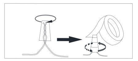
Connect the neutral fixture wire to the neutral J-Box wire first and then connect the Hot fixture wire to the hot J-Box Wire. Wrap these connections with electrical tape
