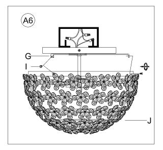
Position the Frame (J) over the Spider (G) aligning the 3 holes on the Spider (G) with 3 holes on the upper ring of Frame (J). Insert 3 Frame Screws (I) and tighten till secure.
