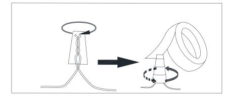
Connect the ground fixture wire to the ground J-Box Wire and wrap the connection with electrical tape
