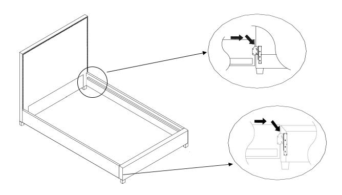
3. Screw support leg (D) onto slat (E) until secure and tight. Lay slats on cleat rail. Using a Phillips head screwdriver and screws provided (G), screw each slat down to the cleat rail until secured.
