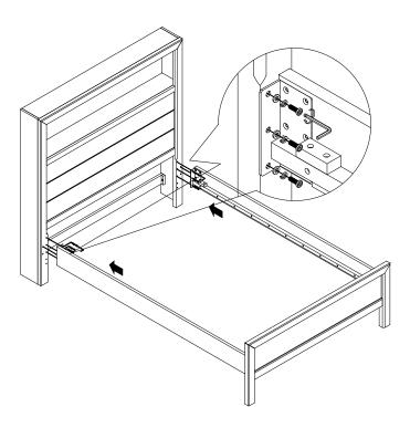
3. Roll out the slat roll of simple base on two side rails and then secure with wood screws (get from simple base box)
