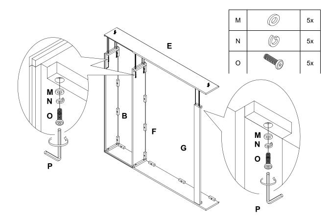
6. Attach the front frame (A) to the wood cleat on the top panel (B), side panels (D,E) and shelf (F), secure with flat washer (M), spring washer (N), short Allen bolt (O) using Allen key (P).
