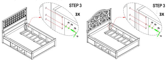
6. Attach a Support side rails (D) to the Side rail (B1) by using Flat Washer (F), Lock Washer (G), and Allen Bolt (H). Tighten with the Allen Key (I), as seen in the illustration below.
