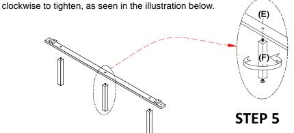
10. Attach Slat (D) to Support slat (E) by using Flat Washer (N), Lock Washer (M), and Allen Bolt (L). Tighten
