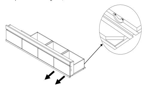
2. Attach Siderail (B2) with Footboard (A) by Flat Washer (F), Lock Washer (G), and Allen Bolt (H). Tighten with the Allen Key (I).
