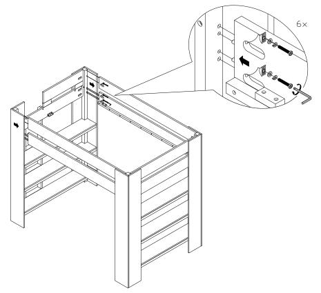
18. Place the center support rail (S) onto the pre-attached metal U bracket on the headboard and footboard panels
