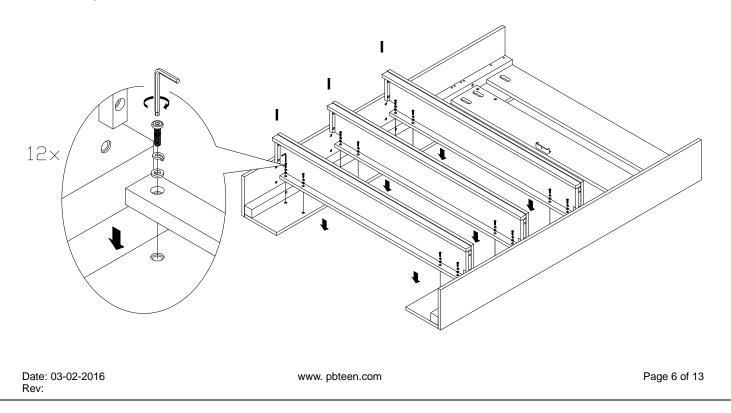
6. Secure the shelves (I) to vertical panels 1 and 4 (C&F) by flat washer, spring washer and short Allen bolt (30 mm) using Allen key.
