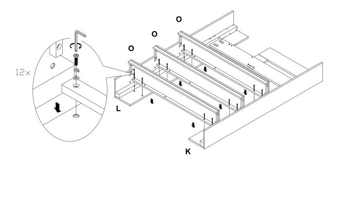
12. Secure the shelves (O) to vertical panels (J&M) by flat washer, spring washer and short Allen bolt (30 mm) using Allen key.
