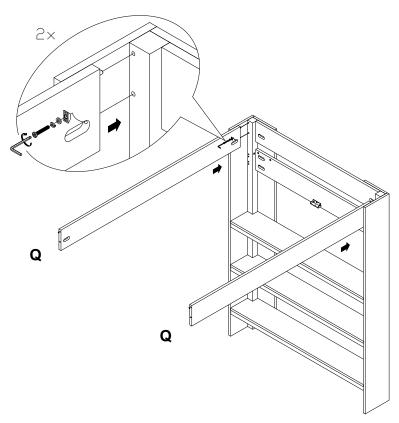
15. Attach the lower side rails (R) to headboard aligning the exposed wood dowel with pre-drilled holes. Secure the lower side rail by fitting, flat washer, spring washer and medium Allen bolt (55 mm) using Allen key as shown
