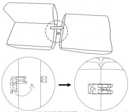
3. To separate the group, just lift the end with **MALE BRACKET**, and then rotate the female bracket back.
