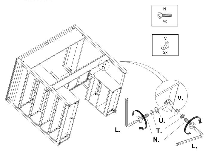
7. Slide a Spring Washer (T) and a Flat Washer (U) onto (3) Medium Bolt (S). Under the desktop, insert (2) Medium Bolts (S) with washers from wooden cleat pre-installed to Center Shelf of the Bookcase into insert nuts located on bottom of the Desktop.
