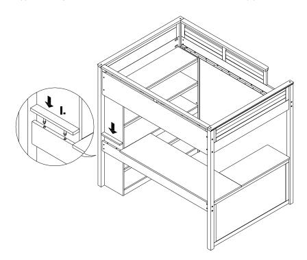
6. Slide a Spring Washer (T) and a Flat Washer (U) onto (4) Short Bolt (N). Align (2) L-Shaped Bracket (V) to pre-drilled holes located on bottom of the Desktop and Footboard Bottom Panel and insert (4) Short Bolts (N) with washers to secure.
