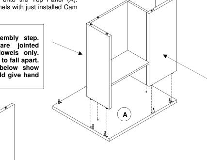
8. Attach the Large Side Panel (C) on the Top Panel (A). Align the dowels on the side with pre-drilled holes on top.
