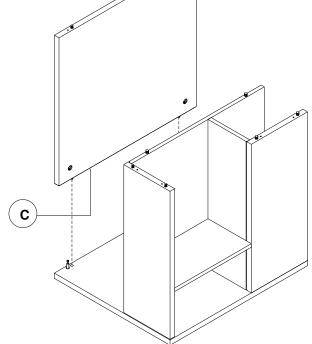
9. Attach the Bottom Panel (B) onto the assembled parts by aligning wood dowels and pre-drilled holes.
