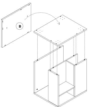
10. Insert the Cam Lock (K) into the pre-drilled hole on Large Side Panel (C), Small Side Panel (D) and Back Panel (E). Two for each panel with the arrow mark on the cam lock turn down at 90 degree with Top Panel (A). This will ensure the head of cam bolt could slot into the cam lock. Tighten Cam
